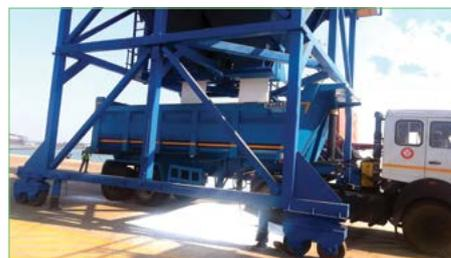
CARGO FALLS INTO A TIPPER FROM THE HOPPER FOR ONWARD MOVEMENT TO A WAREHOUSE
