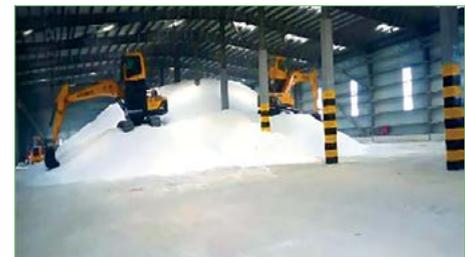
EXCAVATORS ARE USED TO MAKE HIGH HEAPS OF BULK CARGO
