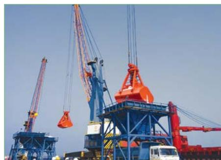
BULK CARGO IS DISCHARGED INTO HOPPERS
