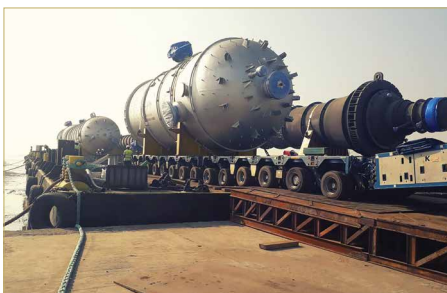
PACKAGES ROLLED ON TO THE BARGE
